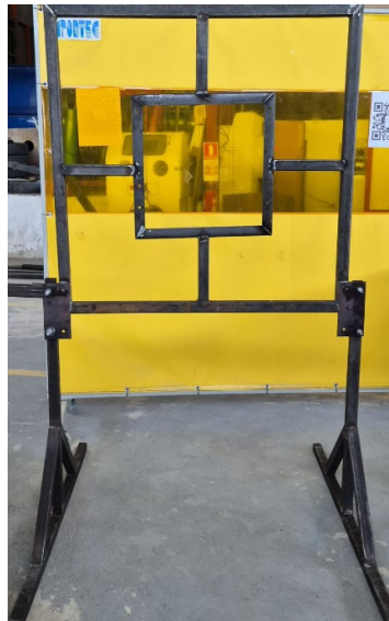
Figure 2. Fabricated plate carrier.
