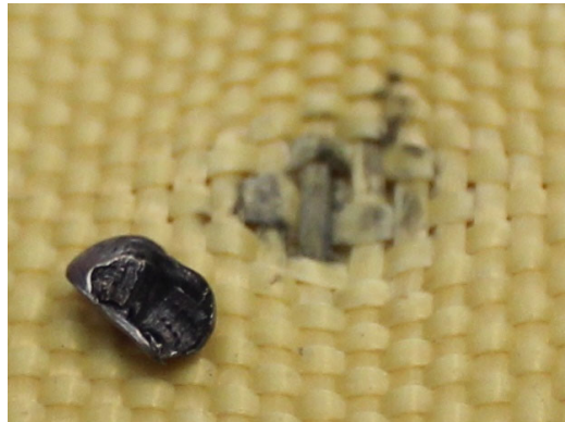
Figure 20. Fragment of the 5.5 mm projectile in layer 5.
